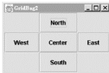
Figure 16.8. Making buttons fill the available space
