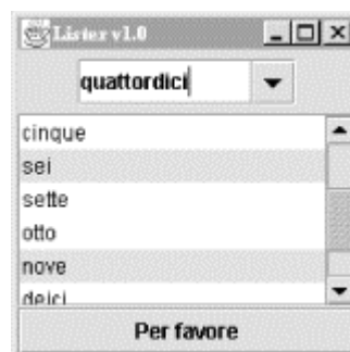
Figure 14.2. A combo box and a list using the same data model
