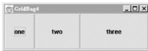
Figure 16.10. Using weight to control component size
